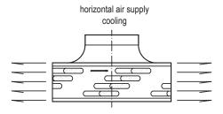
VENTILATION – in case the air-supply has the same temperature as the air in the room, a mixed air-supply must be utilised. In this way, the air is supplied horizontally and vertically, which enables it to reach as much space of the room as possible.
